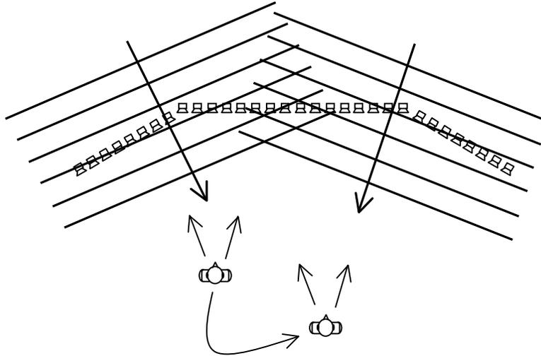
**Fig. 6 - Realization of a virtual scene presenting a compatibility with stereophony 2-0.0 by means of virtual plane waves. The two auditors perceive the same directions of incidence.**
