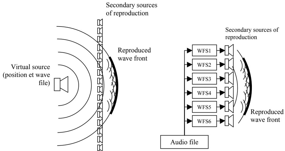
**Fig. 4 – On left, the principle of construction of Huygens applied to the reproduction. On right, a simplification of the realization of WFS for a single virtual source.**
